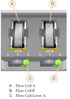
Figure 3 Flow Cell Stage With High Output Flow Cells
