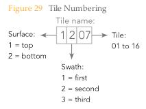
This example indicates a tile from the top surface of the flow cell, the second swath, and the seventh tile.
