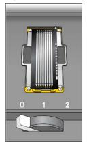
4 Lift the used flow cell from the flow cell holder.
