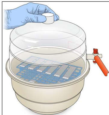
Figure 55 Testing Vacuum Seal
