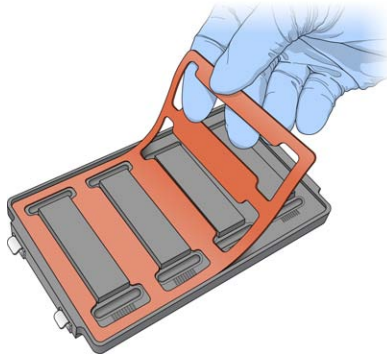
Figure 31 Placing Gasket into Hyb Chamber
