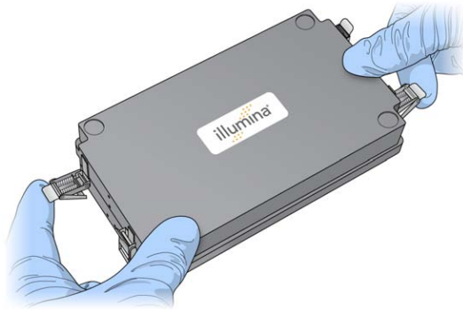
Figure 34 Sealing the Hyb Chamber
