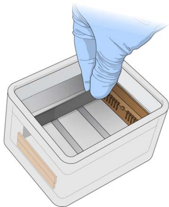
Figure 42 Submerging BeadChips in Wash Dish Containing E1BC Buffer
