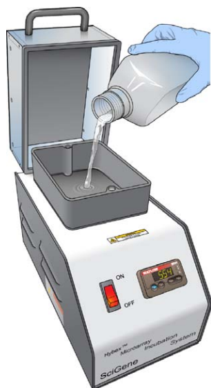
Figure 39 Adding High-Temp Buffer to Hybex Waterbath Insert
