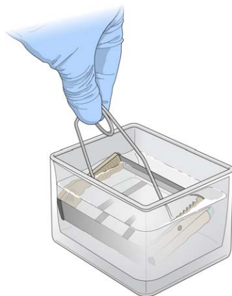
Figure 45 Washing BeadChip in Diluted Wash E1BC Buffer
