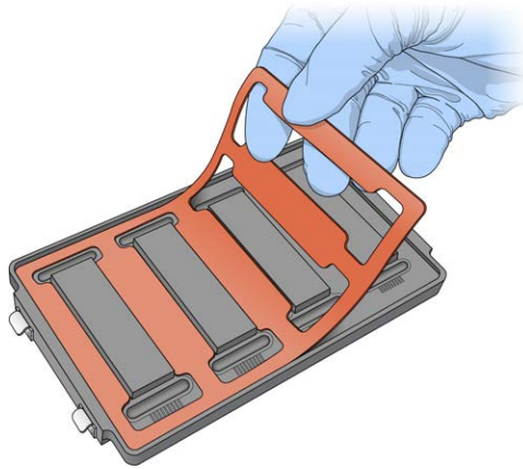
Figure 28 Placing Gasket into Hyb Chamber
