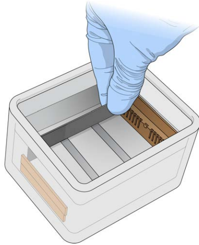
Figure 115 Submerging BeadChips in Wash Dish Containing PB1
