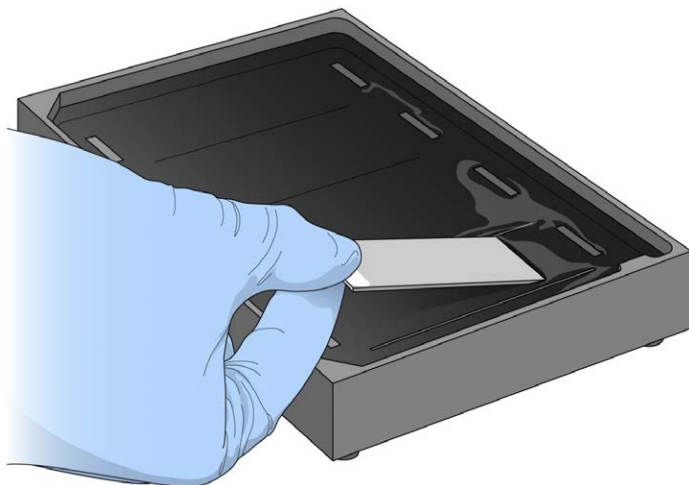
Figure 47 Placing BeadChip into Black Frame on Alignment Fixture
