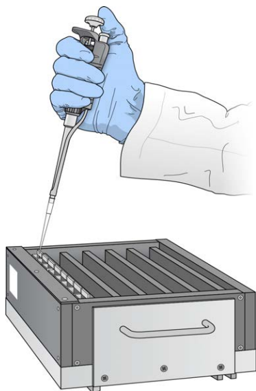
Figure 57 Dispensing RA1 into Each Flow-Through Chamber
