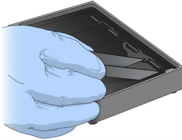
Figure 117 Placing Black Frames into BeadChip Alignment Fixture
