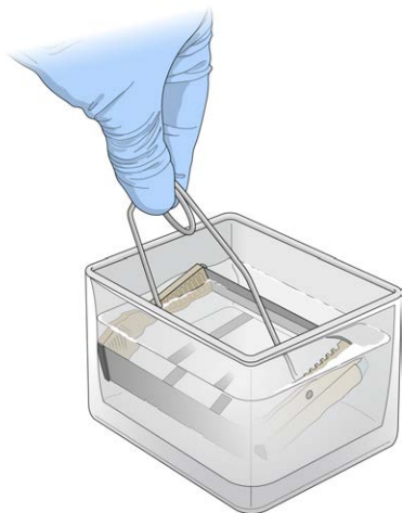
Figure 42 Wash Rack in Wash Dish Containing PB1
