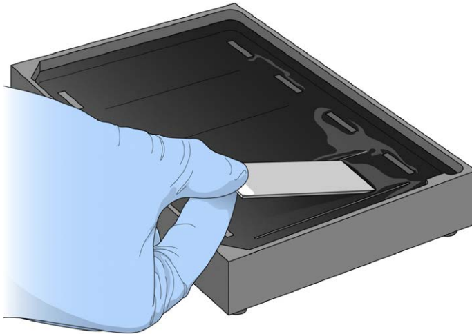
Figure 118 Placing BeadChip into Black Frame on Alignment Fixture
