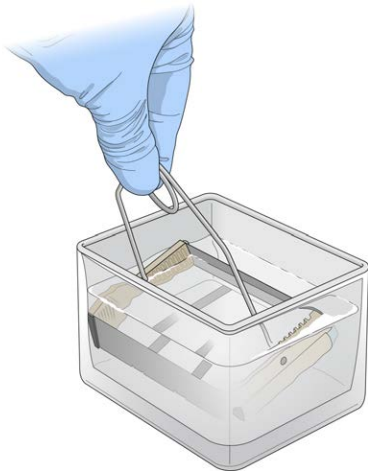
Figure 113 Wash Rack in Wash Dish Containing PB1
