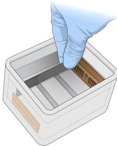
Figure 44 Submerging BeadChips in Wash Dish Containing PB1
