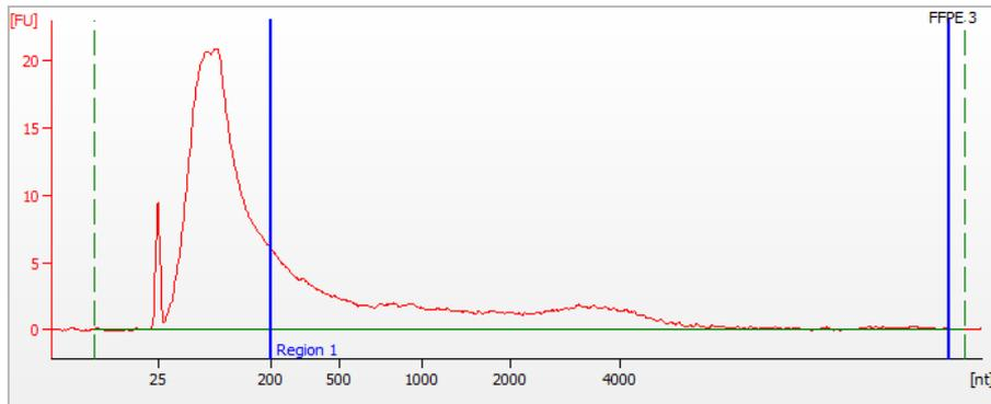
**Figure 5** Example: FFPE Quality Not Recommended for Use ( $DV_{200} = 8\%$ )
