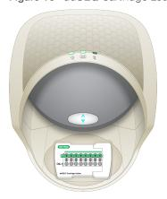
3 Press the silver button on the top of the ddSEQ Single-Cell Isolator to close the instrument . Single-cell isolation begins automatically after the ddSEQ Single-Cell Isolator door is closed and takes approximately 5 minutes. The droplet indicator flashes green to indicate that cell isolation is in progress. Single-cell isolation is complete when all 3 indicator lights are solid green.
