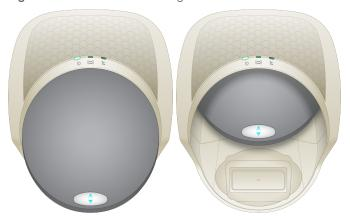
2 Place the cartridge holder into the instrument. Make sure that the cartridge indicator light is solid green to confirm that the cartridge holder is in the correct position. If the cartridge indicator light is not lit, reseat the cartridge holder on the magnetic plate.
