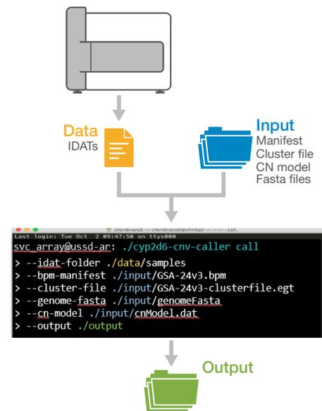
Figure 1: *CYP2D6* CNV Caller workflow—Array scanner data and auxiliary files are input to the algorithm, which outputs CNV calling results.
