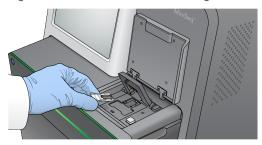
6 Close the flow cell latch to secure the flow cell.
