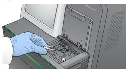
Figure 12 Place Flow Cell on Stage
