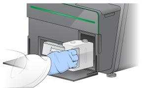
2 To prevent spills when carrying the spent reagents bottle, seal the bottle opening with the threaded cap.
