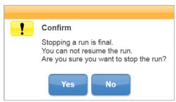
Stopping a run is final. A stopped run cannot be resumed. The only option is to proceed to an instrument wash.
