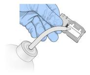
4 Using care around the black flow cell port gasket, thoroughly dry the flow cell and cartridge with a lint-free lens cleaning tissue. Gently pat dry in the area of the gasket and adjacent glass.
