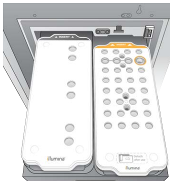
Figure 25 Loaded Reagent Cartridges
