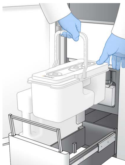
Figure 26 Load the Buffer Cartridge
