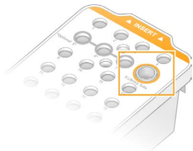
Figure 21 Uncapped Library Tube Loaded Into Position #8
