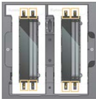
Figure 17 Loaded Flow Cells Aligned Over Clamps
